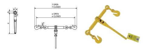
GRADE 70 LASHINGS & FITTINGS ARE NOT TO BE USED FOR LIFTING PURPOSES \* NOTE: The use of some grab hooks or systems incorporating grab hooks cause bending to occur on the link of lashing chain to which the grab hook is engaged. The bending and shearing effect of the hook reduces the strength of the chain by 25 percent and as such, the lashing capacity [LC] of this type of system must be reduced by 25 percent as prescribed in Australian Standard AS/NZS 4344 ഗ
