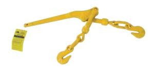
GRADE 70 LASHINGS & FITTINGS ARE NOT TO BE USED FOR LIFTING PURPOSES \* NOTE: The use of some grab hooks or systems incorporating grab hooks cause bending to occur on the link of lashing chain to which the grab hook is engaged. The bending and shearing effect of the hook reduces the strength of the chain by 25 percent and as such, the lashing capacity [LC] of this type of system must be reduced by 25 percent as prescribed in Australian Standard AS/NZS 4344
