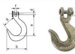
GRADE 70 LASHINGS & FITTINGS ARE NOT TO BE USED FOR LIFTING PURPOSES \* NOTE: The use of some grab hooks or systems incorporating grab hooks cause bending to occur on the link of lashing chain to which the grab hook is engaged. The bending and shearing effect of the hook reduces the strength of the chain by 25 percent and as such, the lashing capacity [LC] of this type of system must be reduced by 25 percent as prescribed in Australian Standard AS/NZS 4344
