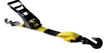
GRADE 70 LASHINGS & FITTINGS ARE NOT TO BE USED FOR LIFTING PURPOSES \* NOTE: The use of some grab hooks or systems incorporating grab hooks cause bending to occur on the link of lashing chain to which the grab hook is engaged. The bending and shearing effect of the hook reduces the strength of the chain by 25 percent and as such, the lashing capacity [LC] of this type of system must be reduced by 25 percent as prescribed in Australian Standard AS/NZS 4344
